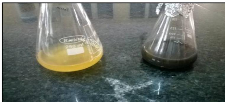
**Fig. 1.**Synthesis of silver nanoparticles from leaf extract incubated with silver nitrate solution
